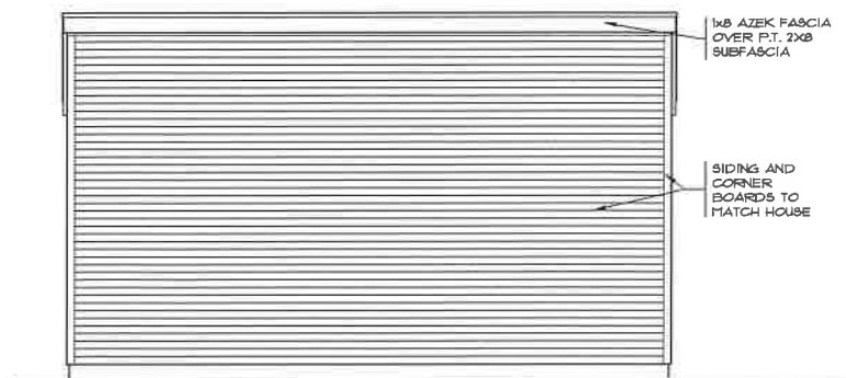
WEST (SIDE) ELEVATION 1/4" = 1'-0"
